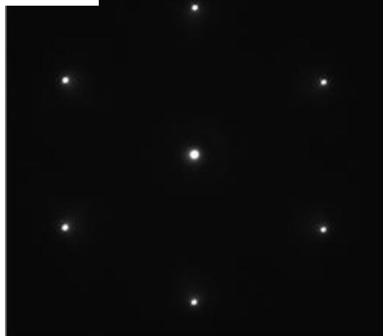
Diffraction patterns of Si [111] (200 keV). www.jeol.co.jp
