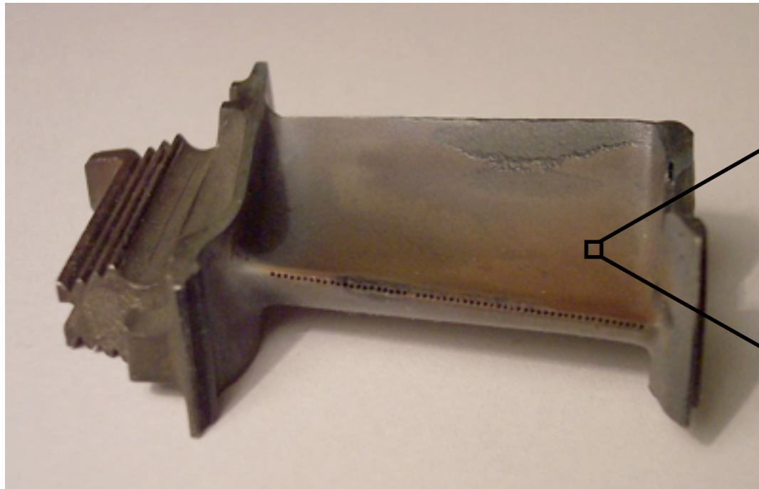
Nickel superalloy jet engine turbine blade
