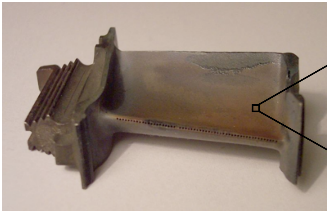
Nickel superalloy jet engine turbine blade
