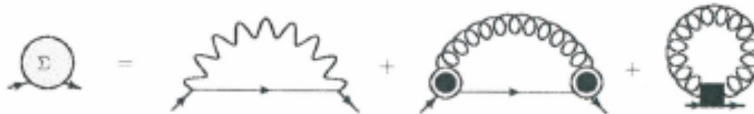
FIG. 10. The Dyson equation at the GW level in the electron-electron and electron-phonon interaction. The electron-phonon diagram is known as Fan self-energy and its vertex (represented by the circled dot) represents a dressed electron-phonon interaction [see Eq. (76)]. The wiggled line is a dressed electron-electron interaction [see Eq. (77)]. The most important aspect of this diagram is that, as long as only skeleton diagrams are included, the second-order electron-phonon interaction, and consequently the DW diagram, is not screened.
