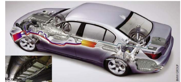
Waste Heat Recovery
