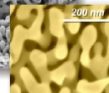
Nanoporous structure: ligaments ~ 30 - 50nm
