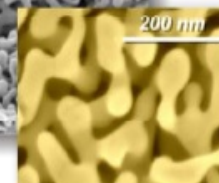
Nanoporous structure: ligaments ~ 30 - 50nm
