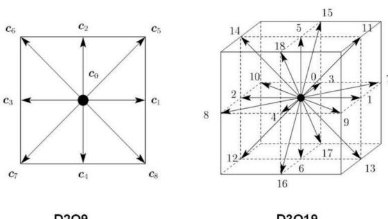
Boltzmann (LB) kinetic model: lattice-based model that simulates the **hydrodynamics** of a liquid and shows excellent scalability on parallel computers. LB is useful in analyzing the hydrodynamics of complex fluids and to deal with suspensions of colloidal particles.
