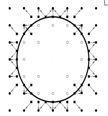
Boundary nodes for a curved surface. The velocities along links are cutting the boundary surface are indicated by arrows. The location of the boundary nodes are shown by solid squares, and fluid nodes by solid circles. The open circles indicate nodes in the solid adjacent to fluid nodes.
