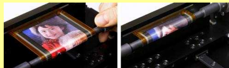
Example: rollable OLED display (Sony, SID-2010)
