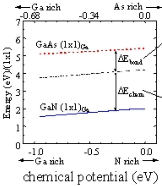
Stronger Ga-Ga bonding (GaN lattice constant 20% smaller than GaAs)
