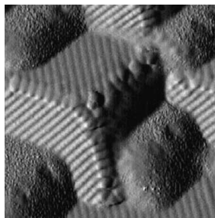
Fig. 17 Atomic resolution STM image ( 10 \times 10 nm) of Pd-covered faceted W(111), prepared by depositing \sim 1.2 ML Pd and annealing at 1075 K. Reprinted from ref. 105 with permission from Elsevier.
