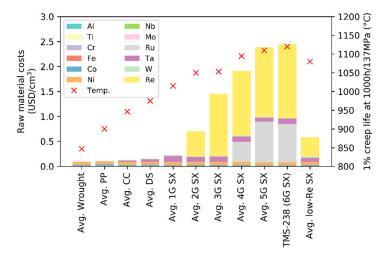
**Figure 2.** Average raw material costs (left-hand scale) and 1% creep life temperature at 1000 h and 137 MPa of each superalloy type (right-hand scale). PP: Powder-Processed. CC: Conventionally Cast. DS: Directionally Solidified. SX: Single-Crystal. Data are in the Supplementary Material (Tables S1 and S5) [2–4,10,28].
