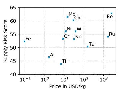
**Figure 4.** Supply risk score on the elemental level and the raw material price in a semi-logarithmic plot. Values are given in Tables S2 and S3 in the Supplementary Material.
