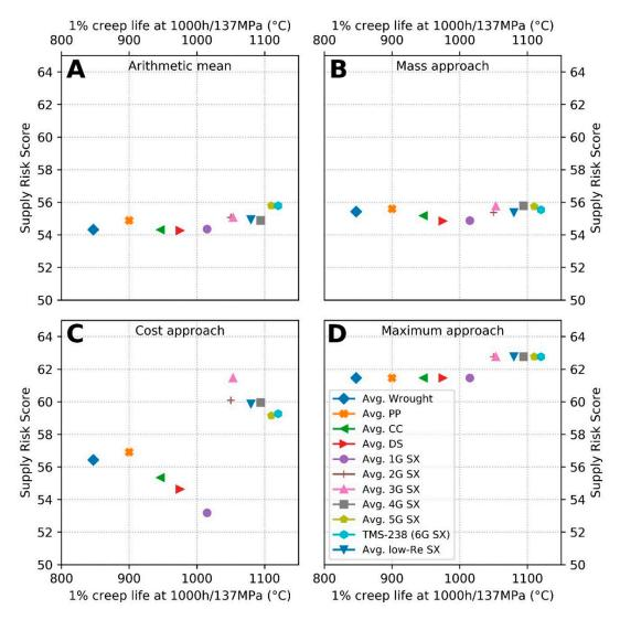
**Figure 5.** (**A**) Supply risk score and endurance temperature on the technology level, using the arithmetic mean as the aggregation scheme. (**B**) Results using the mass approach. (**C**) Results using the cost approach. (**D**) Results using the maximum approach. Raw data are given in Tables S1 and S6 in the Supplementary Material.
