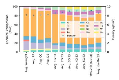
**Figure 1.** Average chemical composition of each superalloy type (left-hand scale) and its density (right-hand scale). PP: Powder-Processed. CC: Conventionally Cast. DS: Directionally Solidified. SX: Single-Crystal. Data are in the Supplementary Material (Tables S1 and S4) [2–4,10,28].
