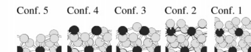
Figure 8. Hard-sphere models of the different surfaces studied to calculate the surface phase diagram (see Figure 7). For each surface, different terminations were possible, leading to the various configurations (geometry optimized structures are shown) shown below each system.
