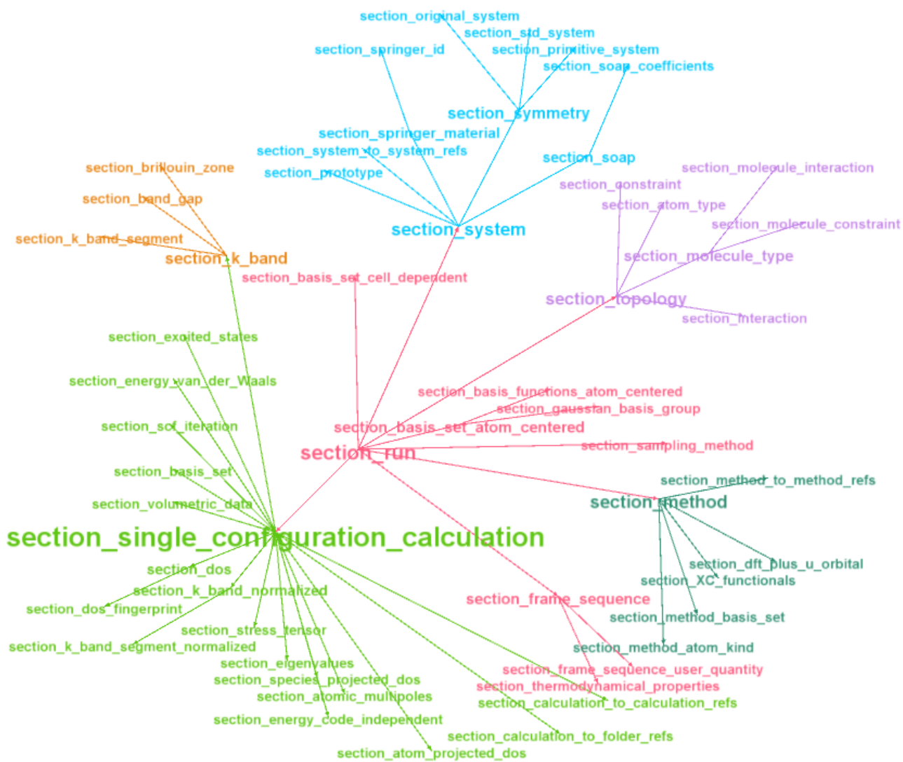
Figure 3.3: Sections in the NOMAD Metainfo represented as network with arrows visualizing the hasSubSection relations. Sections are grouped into communities using the modularity measure. Labels are size-scaled by out-degree. Note that the highest level section is section_run here. Any meta-data concerning the NOMAD entry are not displayed for simplicity.
